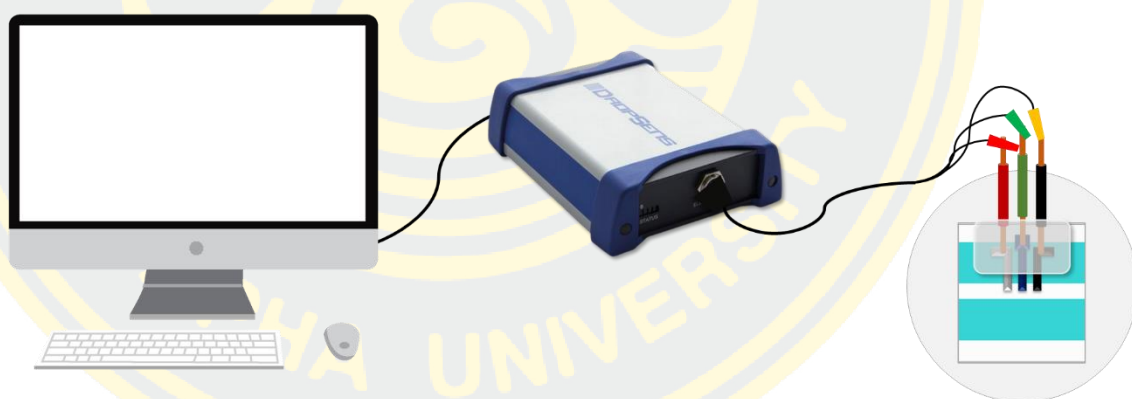
Figures 3-3 Cyclic voltammetry measurement of the electrodes on the cloth-based devices.
